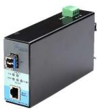
Model SC09FE provides a cost effective plug-and-play solution for long-range 10Base-T or 100Base-TX Ethernet extensions. It has an added benefit of 10/100 auto-negotiation, making it the perfect choice when planning future upgrades of 10Base-T networks. Built-in auto-sensing capabilities enable full or half-duplex Ethernet operation with no configuration required.
